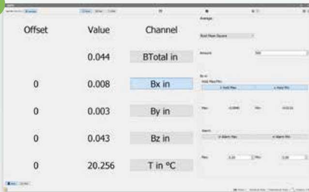
A: Graphical visualization of the measured data ( B_x , B_y , B_z , B_{total} , T ); B: Numerical presentation of the measured data ( B_x , B_y , B_z , B_{total} , T ), as well as Hold function, B_{min} , B_{max} data and alarm function
