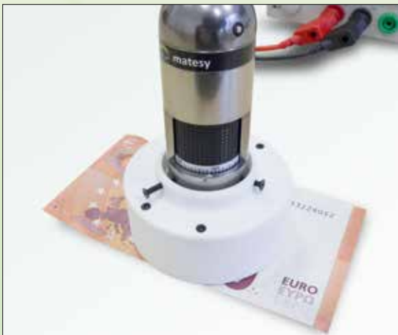
Visualization of magnetic security features on banknotes with optional yoke
