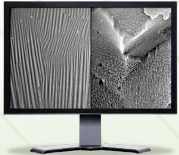
Visualization of domains in electrical steel plates
