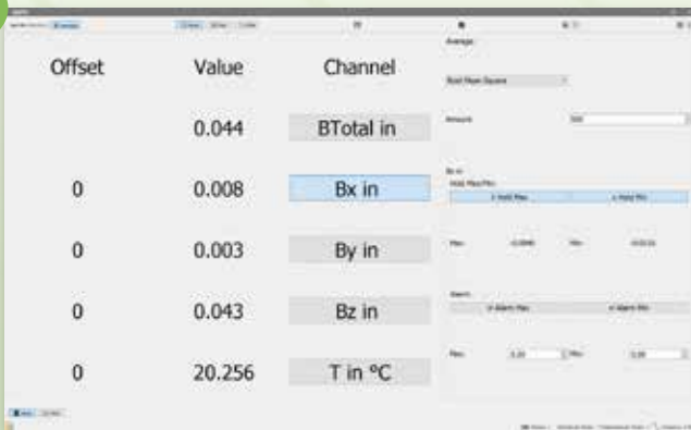
A: Graphical visualization of the measured data ( B_x , B_y , B_z , B_{total} , T^\circ ); B: Numerical presentation of the measured data ( B_x , B_y , B_z , B_{total} , T^\circ ), as well as Hold function, B_{min} , B_{max} data and alarm function
