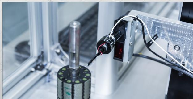
However, in real world the magnetic field is influenced by the quality of the used magnets, a factor which is often not controlled to apply to FEM specifications. The RMP uses Hall probes (single and 3-axial) for absolute and precise flux density measurements. The chucks can be exchanged quickly and easily. It is possible to realize every requirement for quality control of various rotors. (Dimensions, true running characteristics, non-magnetic chucks, etc.)
